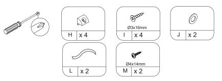
Secure back panel fastener H to the back panel using screw I, then install the anti-tip device on panels 4 and 6
