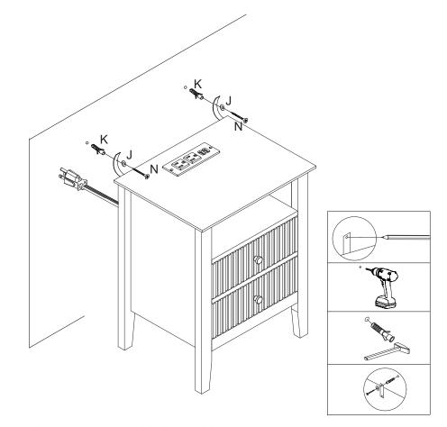
Use components K, J, and N to assemble hardware L on the wall to prevent tipping.
