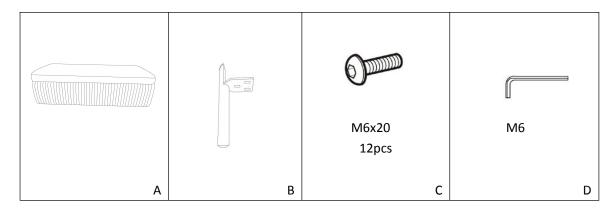
Note: Put all the screws into the hole site, And then tighten them. Do not tighten one by one
