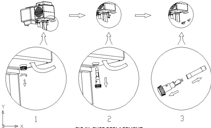
FIG IX: FUSE REPLACEMENT
