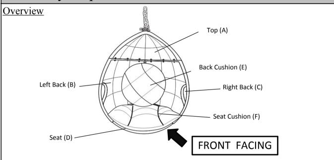
This Basket has multiple parts and may require up to 30 minutes to assemble. The above picture is to help you put the various parts into perspective. Please read through the instructions below to familiarize yourself with the parts and steps before assembly.
