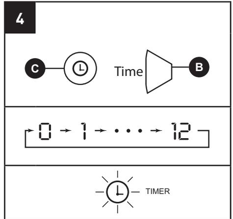
11. To set the timer to power on the heater, first ensure the unit is powered off, then press the timer button on the control panel (C).
