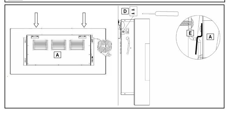
**STEP 5. A.** With the help of a capable adult, lift the fireplace (A) and align the hooks on the back of the fireplace with the slots on the wall bracket. Carefully set the hooks into the slots.
