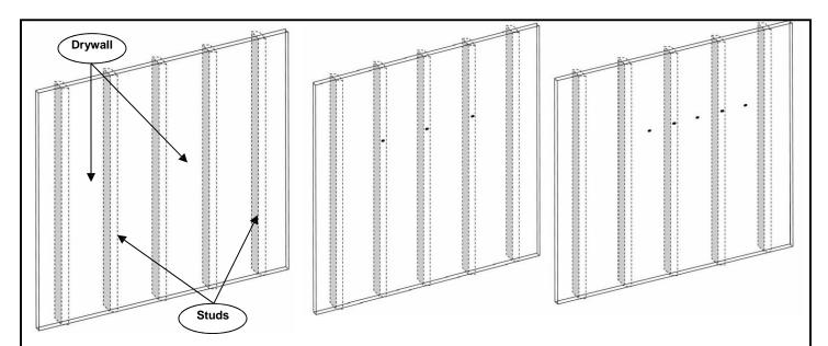
**STEP 2. A.** Locate the wall studs using an electronic stud-finder. Mark the hole locations with a pencil. The holes should be 8" (20.3 cm) apart, and level. The minimum height from the surface below must be 19.7" (50 cm). **B.** Three screws should be screwed directly into wall studs. Then, no drywall anchors are needed. **C.** If only two studs are available, two screws MUST be screwed directly into studs, and the other screws must be screwed into the drywall anchors.
