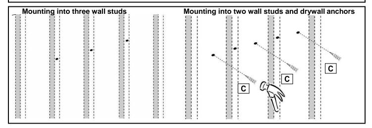
**STEP 3.** Drill a pilot hole into each mark using a 1/4" wood drill bit. **A.** If screws will go into three studs, no drywall anchors are needed. **B.** Tap the drywall anchor(s) (C) carefully into the drywall holes until they are flush with the drywall surface. Use care to avoid damage.
