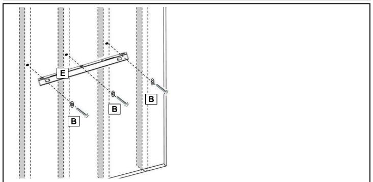
**STEP 4.** Align the holes in the wall bracket (E) with the pilot holes and drywall anchors. Thread wood screws (B) through washers and holes in the wall bracket, then directly into the wall studs and/or drywall anchors. Make sure bracket is level. Tighten all screws securely with a screwdriver.
