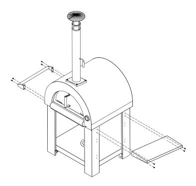
Installed handle and side table as showed. \*Both left and right side can mount side table.
