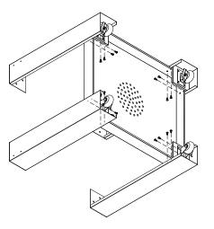
2/. Fasten legs on the oven body with 12pcs of 1/4"\*15mm screws
