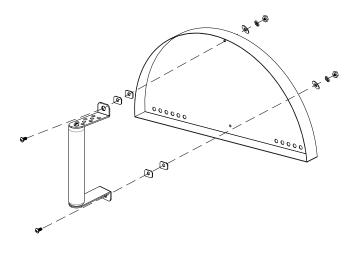
7/. Installed Chimney with 4pcs of 1/4"\*15mm screws
