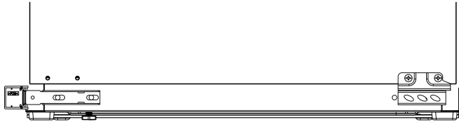
The lower part of the fixed foot and fixed foot pad is installed
