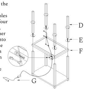
Add another layer of the LED module with glass (F) and another layer of poles (D) by using the two-sided bolts (E). Then, plug in another connector from the power cord (G) into the back of the LED module (F).
