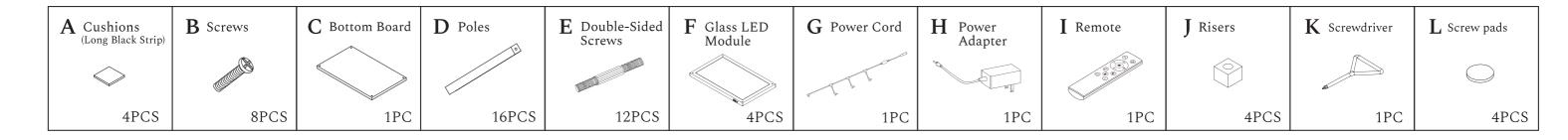
Insert screws (B) all the way through the squared risers (J) and bottom board (C) with the sticker side facing down. Tightly twist four poles (D) clockwise to where the screws emerge on the other side of the board (C) until tight. Use screwdriver (K) if needed to hold the screw while twisting. Place cushions (A) to cover the holes if necessary.
