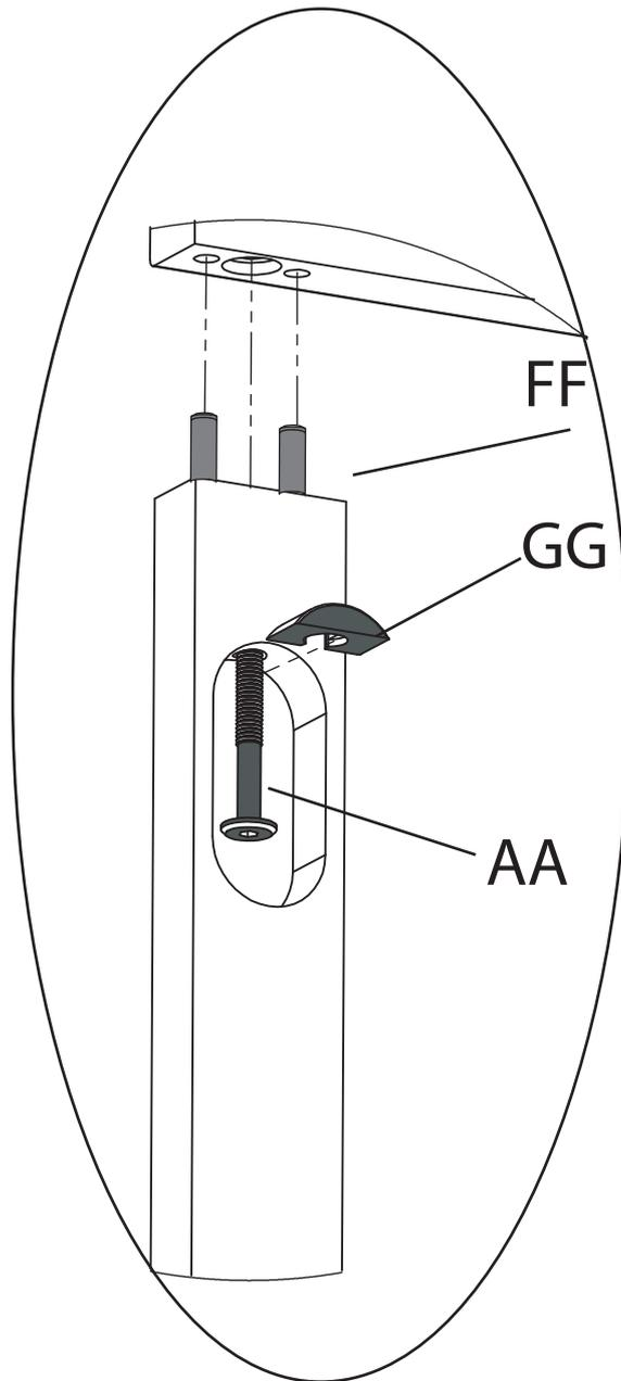
Attach the Right Side by aligning the Right Side (Part B) with the installed Dowels from the previous step and using (4) 60mm Bolts (Part AA), (4) Plastic Clamp (Part GG) and (2) 25mm Bolts (Part DD) following the direction on page 5. Tighten all bolts with the Hex Wrench.
