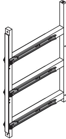
Insert the Divider Frame (Part H) into the (2) Middle Front Rails and Bottom Back Panel using (6) 8mm Dowels (Part FF), (1) 50mm Bolt (Part CC) and (3) 30mm Bolts (Part BB). Tighten all bolts with the Hex Wrench.
