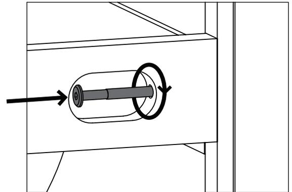
3. Slide the Plastic Crescent Washer over the exposed bolt, behind the head of the bolt. Tighten the bolt with the M4 Hex Wrench Screwdriver provided.
