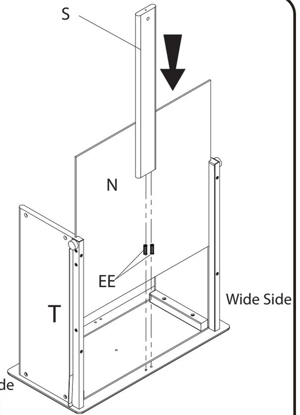
Slide Drawer Bottom (Part N) into the grooves. Install the Drawer Support (Part S) using (2) 6mm Dowels (Part EE).
