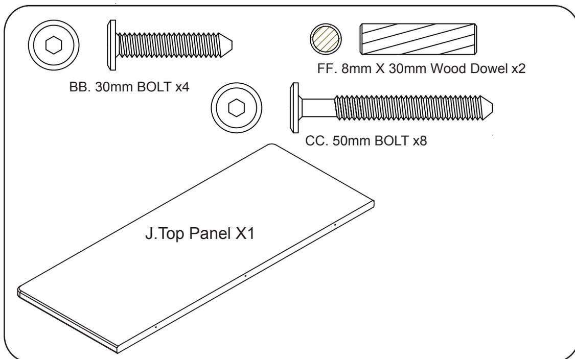
Attach the Top Panel (Part J) to the Case using (2) 8mm Dowels (Part FF) (8) 50mm Bolts (Part CC) through the Top Front and Back Rails, then install (4) 30mm Bolts (Part BB) through the sides. Tighten all bolts with the Hex Wrench.
