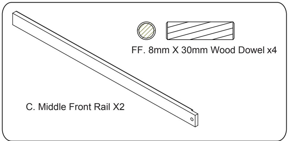
Install (2) Middle Front Rails (Part C) using (4) 8mm Dowels (Part FF).
