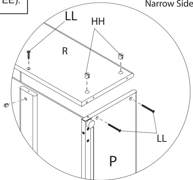
Install the Drawer Support (Part S) and Drawer Back (Part R), using (5) 40mm Screws (Part LL) and (5) Plastic Barrel Nuts (Part HH). Note: Grooves In Bottom Must Align. Tighten All Screws With Phillips Screwdriver.
