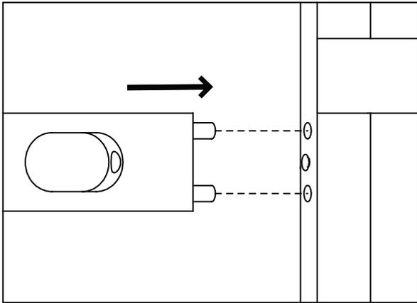
2. Align the bolt with the hole in the end of the rail, align the dowels in the end of the rail with the with the holes in the post. Slide together until tight.
