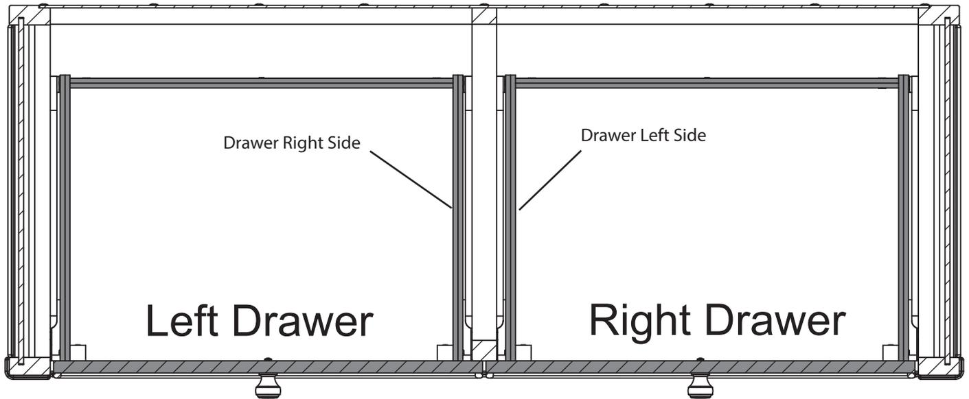
View from above of correctly assembled and installed drawers, the top and top front rail have been removed for clarity.
