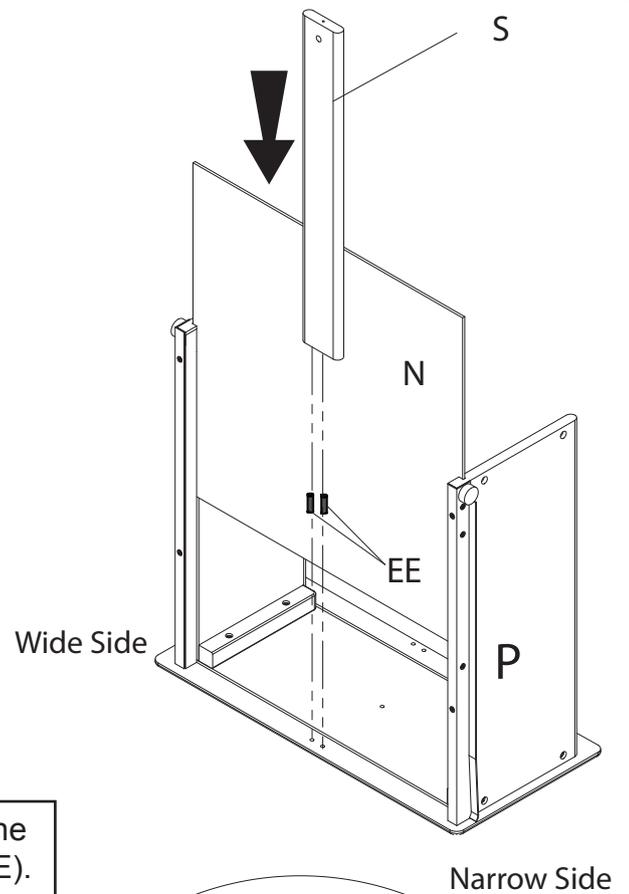
Slide Drawer Bottom (Part N) into the grooves. Install the Drawer Support (Part S) using (2) 6mm Dowels (Part EE).
