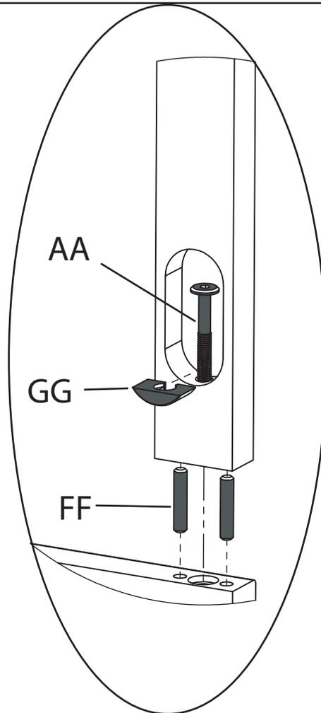
Attach Top Front Rail (Part D), Bottom Front Rail (Part E), Top Back Rail (Part F) and Bottom Back Rail (Part G) to Left Side (Part A) using(8) 8mm Dowels (Part FF), (4) 50mm Bolts (Part CC) and (4) Plastic Clamps (Part GG)following the direction on page 5. Ensure that the slots on the rails face the inside.
