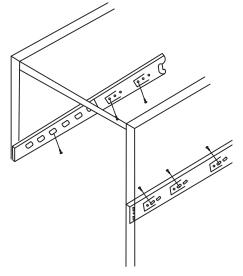
④ Align the track holes with the cabinet holes and screw in the screws to fix
