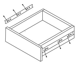
3 Align the position of the slide rail hole with the hole position of the drawer, and screw in the screws to fix
