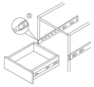
⑤ Align and install the guide rails on the drawer into the guide rails on the cabinet to complete the installation
