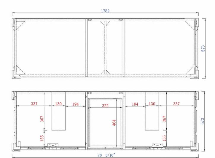
NOTE ONE: Countertops are not shown in these diagrams. (Cabinet Only) NOTE TWO: Wooden Backsplash (Shown) is designed for the molding detail
