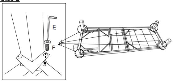
Attach Front and Back Legs(C) to the Seat Panel(A) using Bolts(F) with Allen Key(E) as pictured above. **Do not fully tighten the Bolts.**
