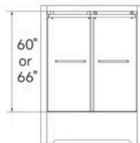
Tub Shower Door
