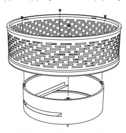
**Step 3**: Put Log Grate (E), Grill (B), Lid (A) on the Fire Bowl (C)Put the Metal Lid (A) on the fire bowl to use as a table. Cover it after the fire pit has completely cooled.
