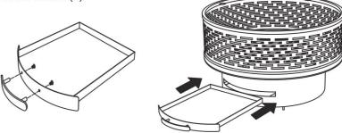
Step 2: Attach Fire Bowl (C) to Base (D) using M6 x 10mm Bolts (BB)×4. Tighten all the hardware.
