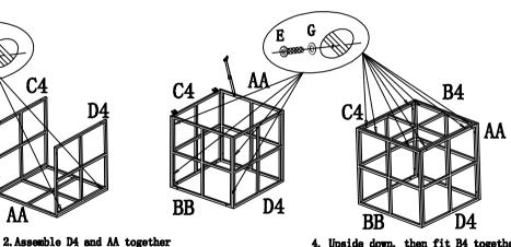
4. Upside down, then fit B4 together with AA, D4, BB, C4, assemble with screw (E), washer(G), total Splaces.
