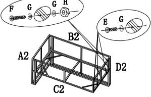
Fit D2 and A2 together by using Fit A2 and B2 together with C2, by using of screw of screw (F), nut (H), washer (G). Total 2places.
