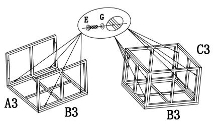
1. Assemble A3 and B3 together with screw (E), washer (G), total 4places. \*Please always do not tighten up the screws in one time before you assemble all the rest parts.
