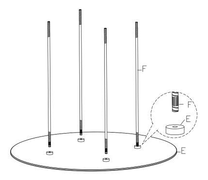
Insert attached long bolts (F) through the corresponding holes on stretchers (A) as shown below.
