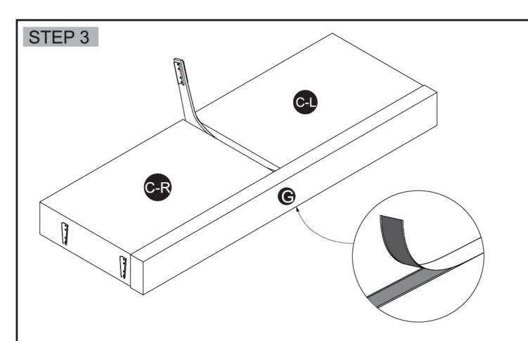
Remove the Velcro from Fabric "G" and attach to the seat frame "C-R" ,"C-L"
