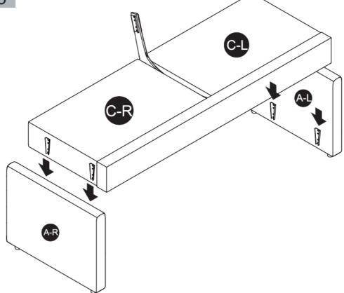
Please put armrests on the ground and lift the seat frame to insert into armrests
