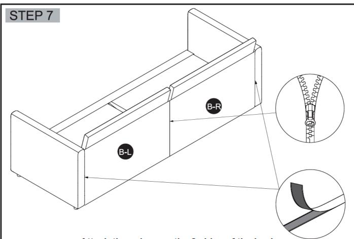
Attach the velcro on the 2 sides of the back and connect 2 back frame by zippering up the center of the back
