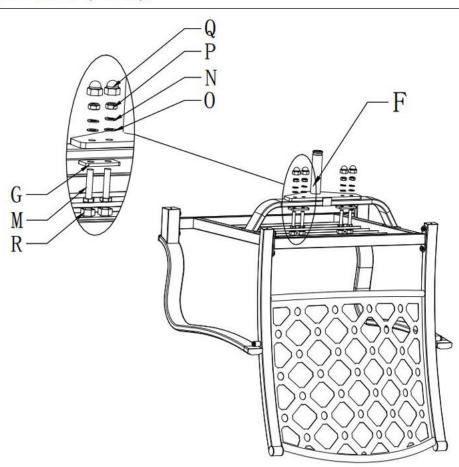
Assembly Part F with the seat (Part C) according to the direction of the picture. Then put on the Part O, Part N, Part P, Part Q and Part G, Screws (Part M). Then cover the lid (Part R). After all the screws are assembled in place, tighten them together.
