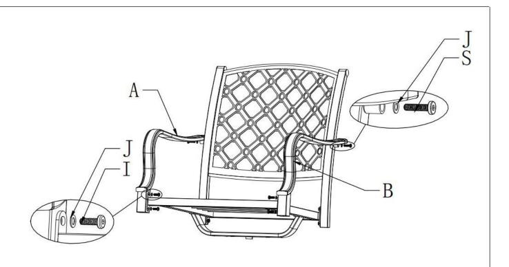
Assemble armrest (Part A & Part B) and the seat(Part C) with Part J and the Screws (Part I). Assemble armrest (Part A & Part B) and the back(Part D) with Part J and Screws (Part S).
