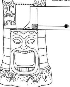
Adjust the pump flow rate to achieve the desired effect and to minimize any splashing. Splashing can occur if the flow rate is too high or the feature water level is too full. The flow rate can be increased or decreased by moving the flow rate control slider on the pump body. Moving the switch towards (+) will increase the flow rate and moving it towards (-) will decrease it.
