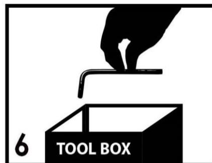
6 Save the instructions and store the Allen wrench or any supplied tool for later maintenance. After two weeks, check and tighten any loose hardware and repeat again every six months thereafter.
