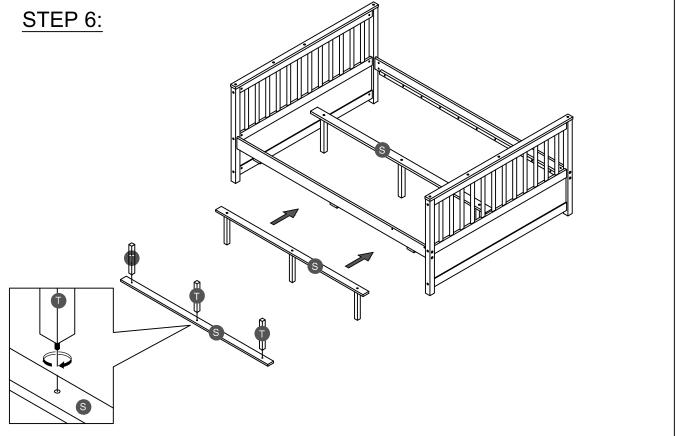
Assembling leg support (T) with lower support slat (S) later rotate, Move support slat inside Full bunkbed.
