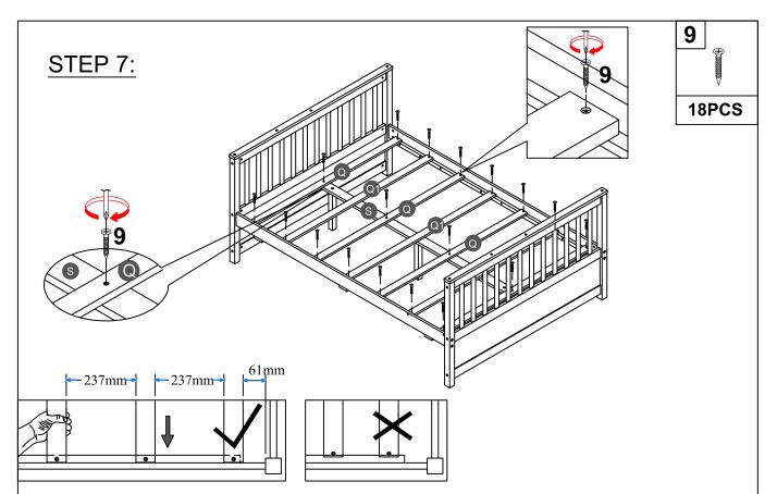
Note: Do not lock the screws of the bed slats to the outermost edge of the bed slats, you need to leave a certain space at the edges, otherwise it will cause the board to break. Do not lock the bed slats on the edge of the wood, please hold firmly before screwing, hold it in place with one hand, then lock the screw.
