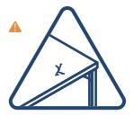
6. Pay attention to avoid over-tightening fasteners, or they may induce cracking within the board.
