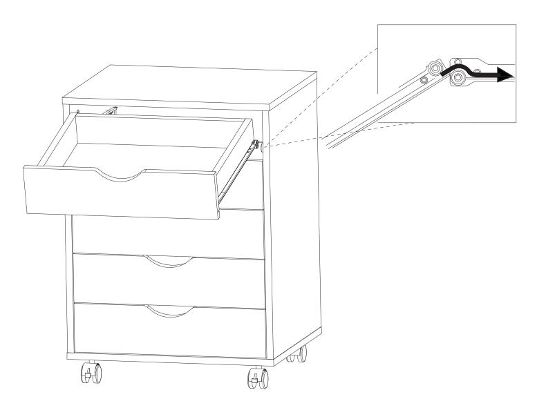
Align the Slide Rail on the Drawer with the unit and push it carefully inside until it stops.
