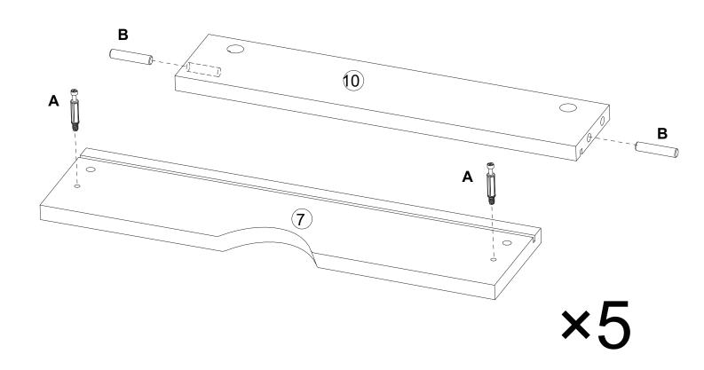
Fix Dowel (A)\*2 to the Board (7). Attach Wooden Dowel (B)\*2 to the Board (10).
