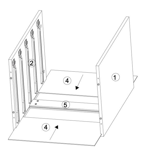
Insert the Boards (4)\*2 into the grooves of the Boards (1&2&5).
