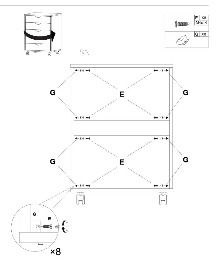
As shown, fix Buckle **(G)\*8** on the back of the installed Cabinet with Screws **(E)\*8**.
