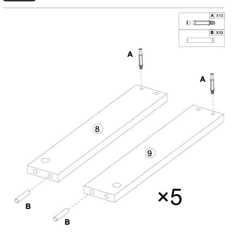
Fix Dowel (A)\*2 to the Boards (8&9). Attach Wooden Dowel (B)\*2 to the Boards (8&9).
