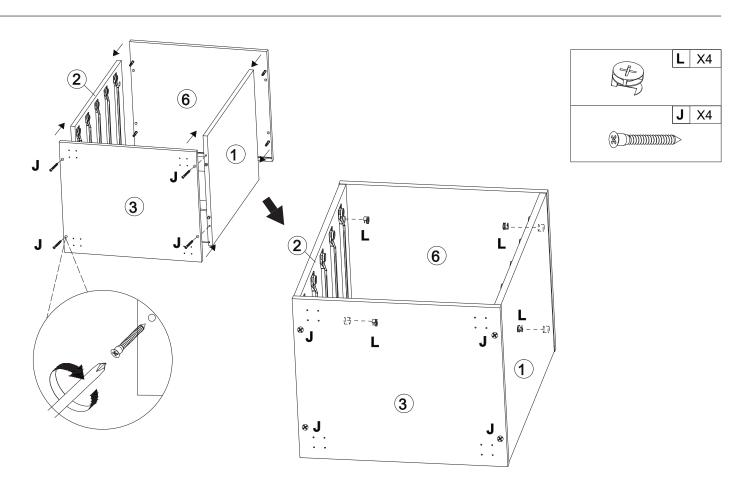
Attach Board (6) to the Top of the Boards (1&2) with Eccentric Wheel (L)\*4. Attach Board (3) to the Bottom of the Boards (1&2) with Screws (J)\*4.
