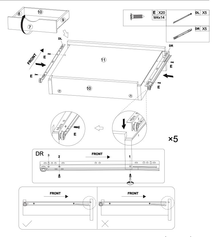
Turn the installed Drawer over. Attach Slide Rails (DL&DR) to the Boards (8&9) on each side of the drawer with Screws (E)\*4.
