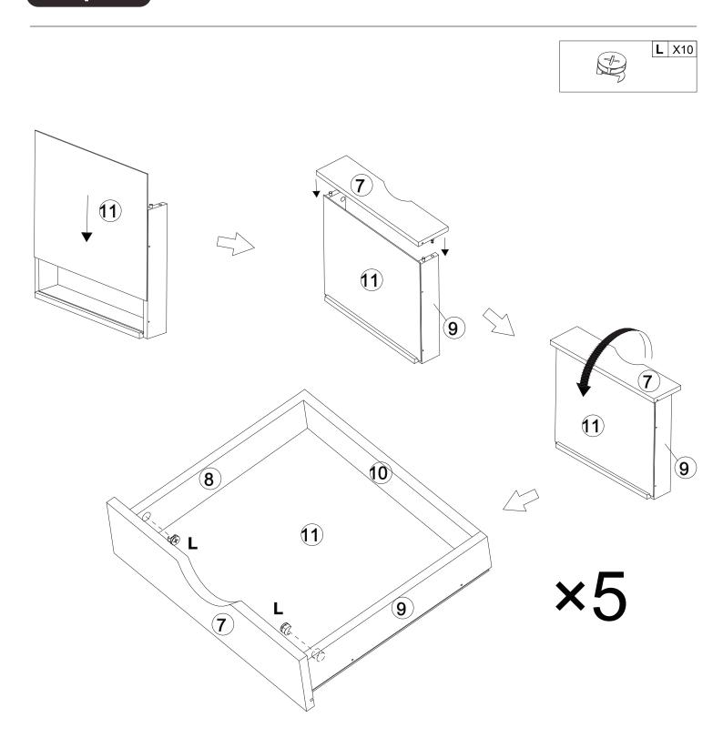
Slide the Board (11) into the installed Board groove. Then fix Boards (8&9) to both sides of the Board (7) with Eccentric Wheel (L)\*2.
