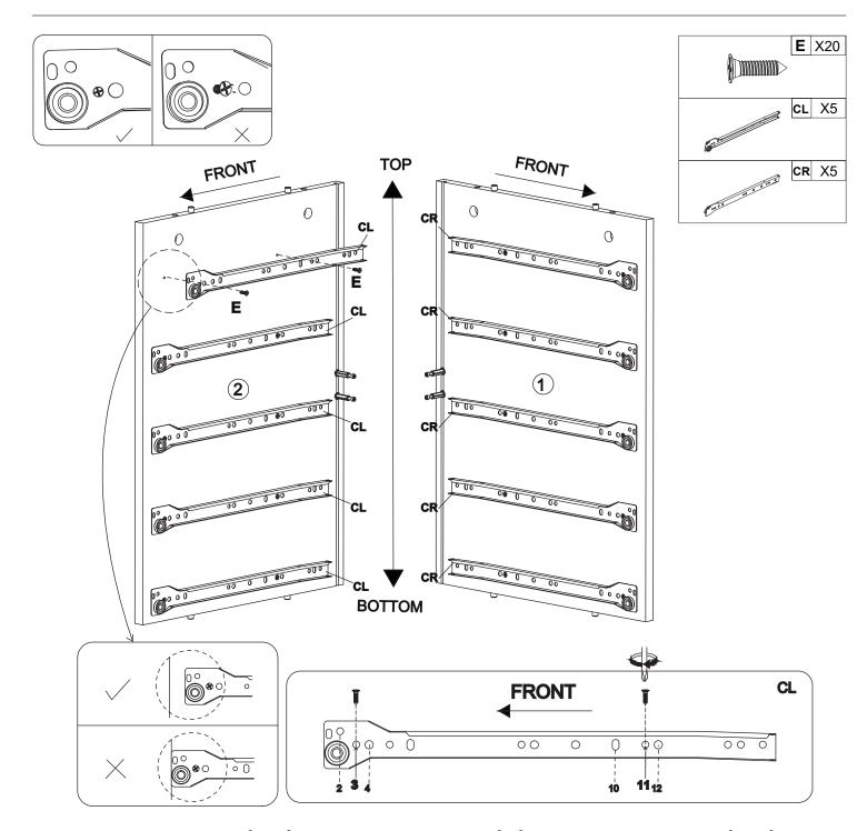
Attach Slide Rail (CL)\*5 to the Board (2), and Slide Rail (CR)\*5 to the Board (1) with Screws (E)\*20.
