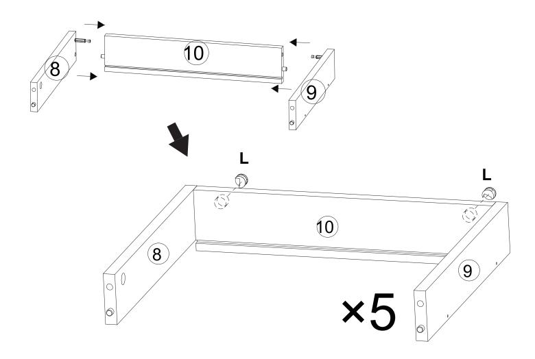
Fix Boards (8&9) to both sides of the Board (10) with Eccentric Wheel (L)\*2.
