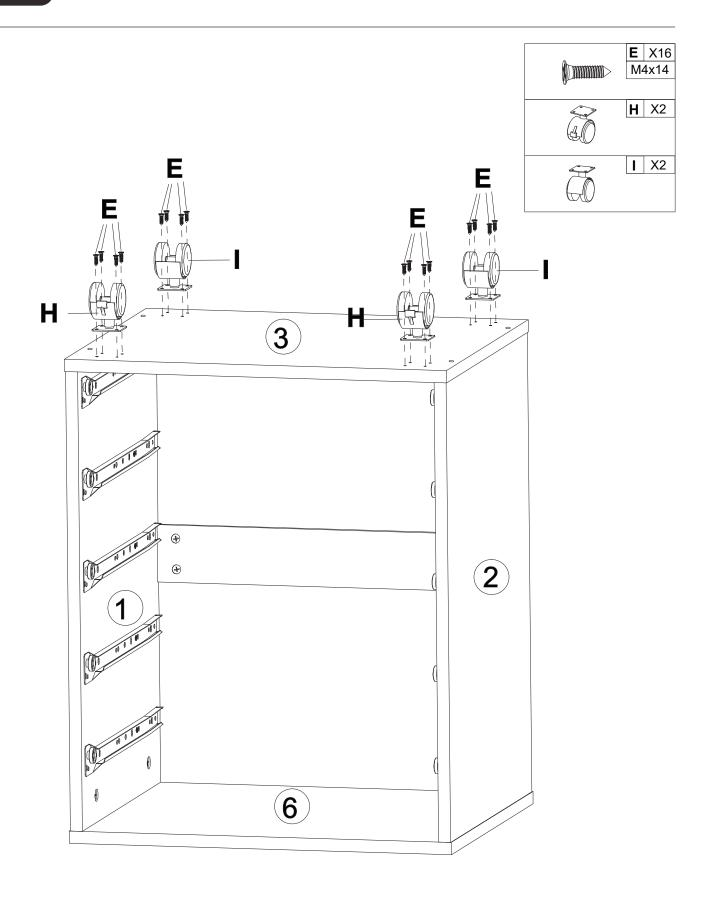
Attach Lockable Casters (H)\*2 to the Front side of the Board (3) and Casters (I)\*2 to its Back side with Screws (E)\*16.
