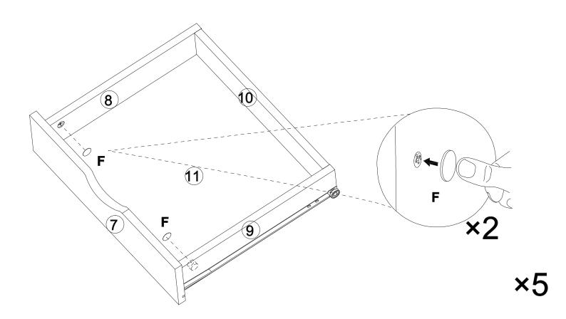
Using Cover-up Sticker (F)\*2 to cover the exposed part of Screws.
