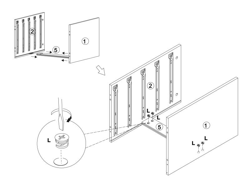
According to the Board position as shown, attach Boards (1&2) to the Board (5) with Eccentric Wheel (L)\*4.
