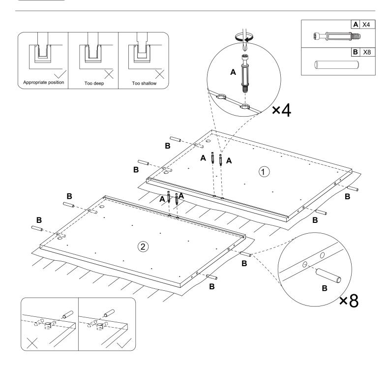
Fix Dowel (A)\*4 to the Boards (1&2). And attach Wooden Dowel (B)\*8 to the Boards (1&2) as shown.
