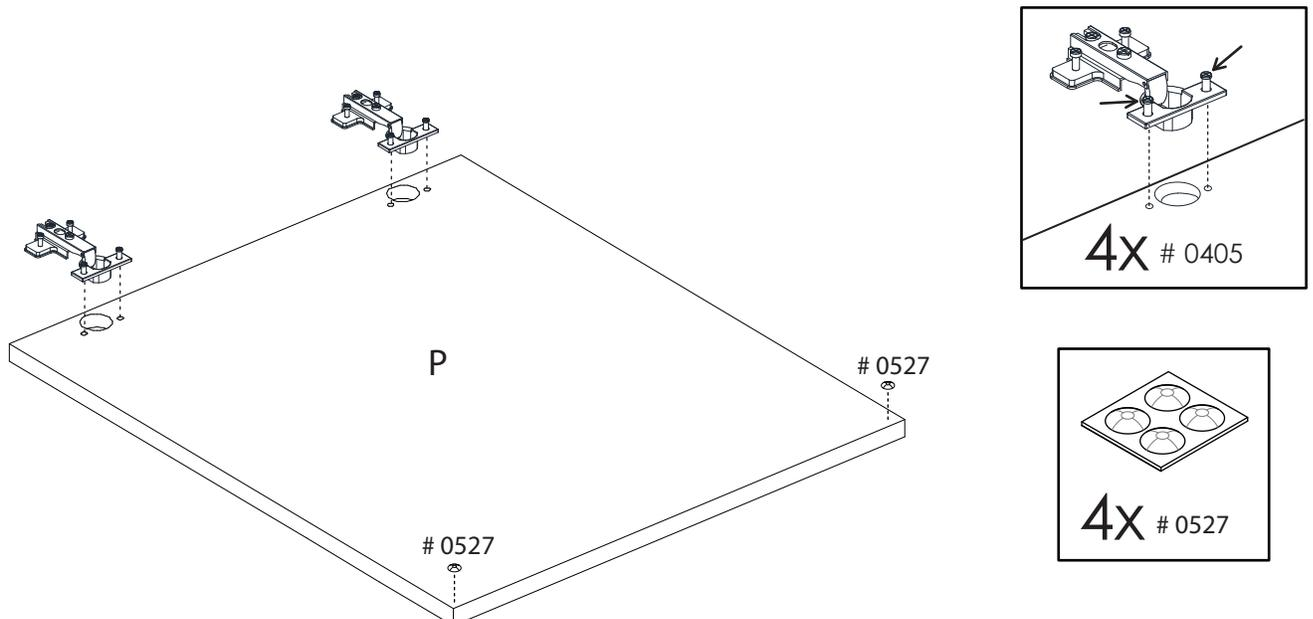
**2** Fasten both doors P to the panels A and B. Then, adjust the 2 doors as shown
