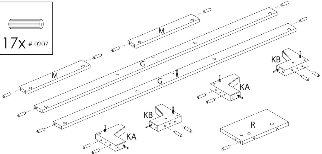
**5** Fasten the panel R to one of the panels G. Then, fasten the 2 panels G to the legs KA and KB. Fasten the 2 panels M to the 4 legs KA and KB. Align the inserted wood dowels to facilitate the assembly. Finalize the step by tightening the 9 cam locks # 0203 located on the panels G, M and R
