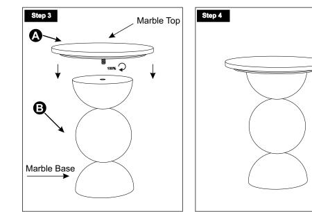
Carefully place the marble top (A) on the marble base (B) and rotate the marble top (A) clock wise.
