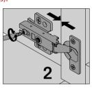
3.Use the screw at the front end of the hinge to adjust the left and right position of the door panel (ensure that the left and right sides of the door panel are in the same plane as the upper and lower panels).
