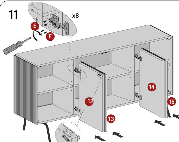
Regarding the installation and adjustment of the door hinge: 1.Use the "waist round hole" marked with a triangle to adjust the position of the door panel(ensure that the gap between the door panel and the
