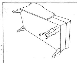
Assemble wooden leg (D) to bottom of seat frame (A) by using screw (4) as shown.
