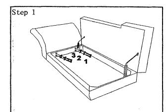
Assemble back (C) to Seat frame (A) by using bolt (1), spring washer (2) and washer (3) as shown.
