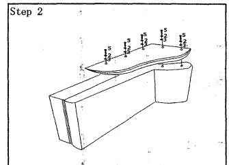
Assemble arm (B) to step 1 assembled unit by using bolt (5), spring washer (2) and washer (3) as shown.
