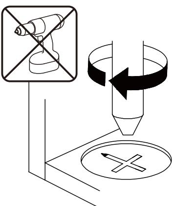
**EN**\_Turn cam lock clockwise to tighten.
