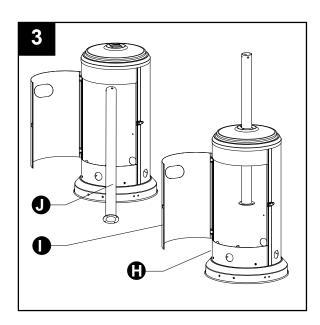
4. Secure post (J) to cylinder housing (H) using the reinforced ring (NN), M6 x 10 mm bolts (DD) and Φ6 small flat washers (EE). Fasten and cover with the deck ring (OO).
