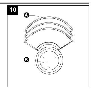
11. Attach reflector panels (A) together using M6 x 10 mm screws (II) and  $\Phi6$  medium washers (HH). Secure loosely with cap nuts (JJ).
