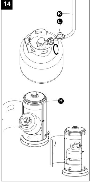
A dented, rusted or damaged propane cylinder may be hazardous and should be checked by your cylinder supplier. Never use a propane cylinder with a damaged valve connection.
