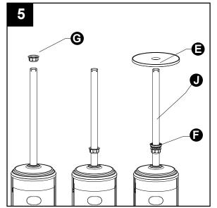
6. Insert the screw coupler (D) on the post (J), inserting it through the middle of the table (E) on the post (J). Thread the tightening spacer (F) on the bottom of the table (E) counterclockwise onto the screw coupler (D). Tighten securely to hold the table (E) to the screw coupler (D). Thread the fastening nut (G) counterclockwise. Tighten securely to lock in place. Loosen the fastening nut (G) to adjust the position of the table (E) on the post (J).
