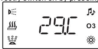
Heating function's model : Long shows is the actual temperature The flicker is the preset temperature
