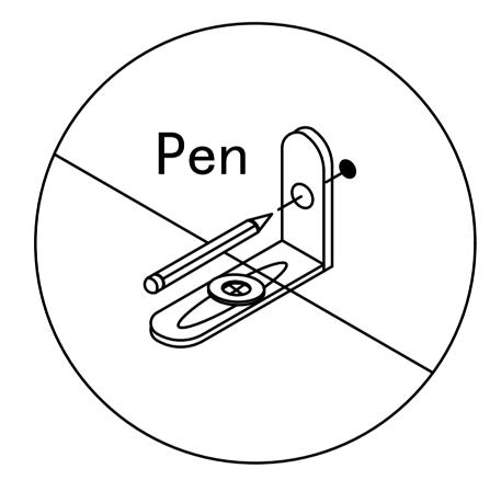
Then mark the wall with a pen through the holes in the
