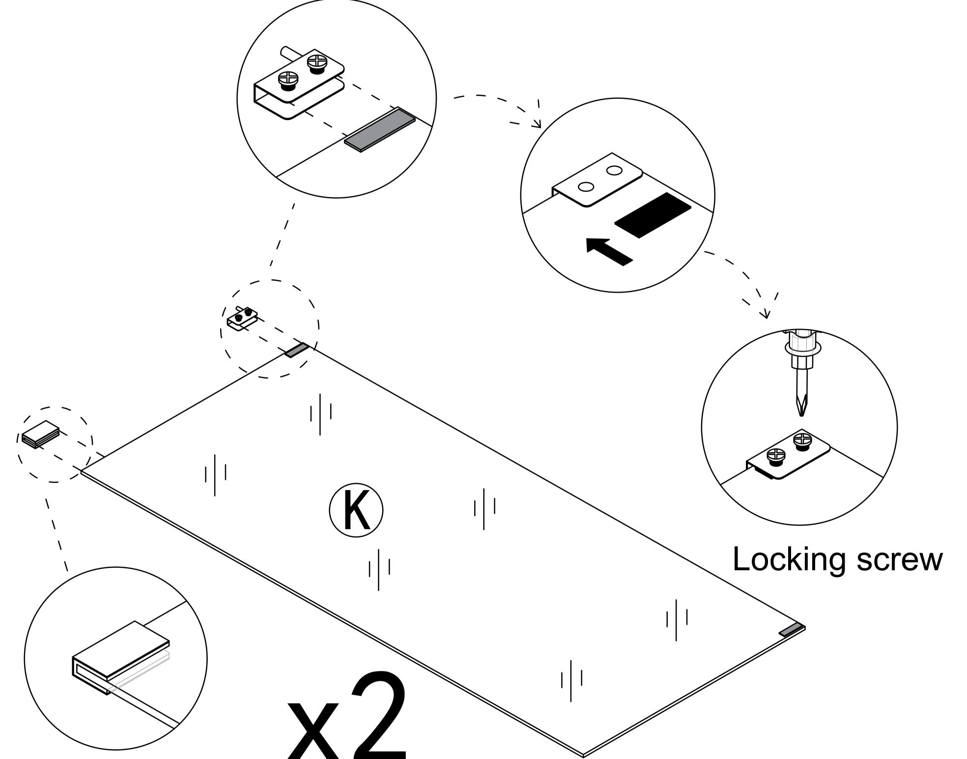
Pay attention to the direction of the door hinge, rotate the screws to compress the black gasket, and do not place it in the opposite direction
