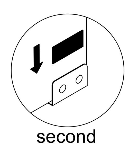
After installing the glass door, place the black gasket on the side where the screws are installed
