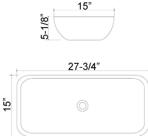
Dimensions of fixture are nominal and may vary within the range of tolerances established by AMSE Standard A112.19.2.2013 Dimensions and specifications subject to change without notice.
