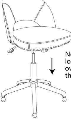
Now turn the assembled seat upright and locate the center hole of the mechanism over the gas lift. Push down firmly until the connection is secure.
