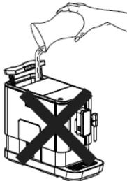
**IMPORTANT: Never fill the water tank with warm, hot, sparkling water or any other liquid which might damage the water tank and the machine. NEVER PUT MILK in the water tank!**
