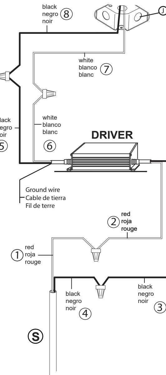
**IMPORTANT: DO NOT ATTACH THE BLACK OR RED WIRES FROM THE FIXTURE STEMS OR DRIVER TO THE SUPPLY WIRES COMING FROM THE JUNCTION BOX. IT WILL DAMAGE THE LEDS AND DRIVER.**
