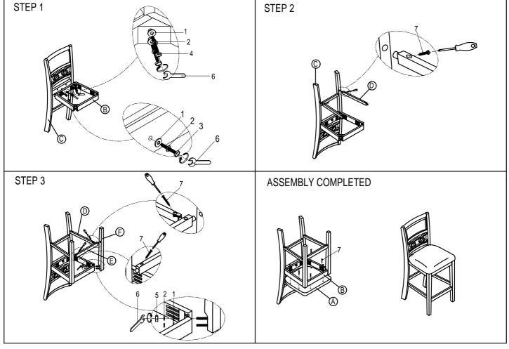
DO NOT TIGHTEN BOLTS UNTIL COMPLETELY ASSEMBLED
