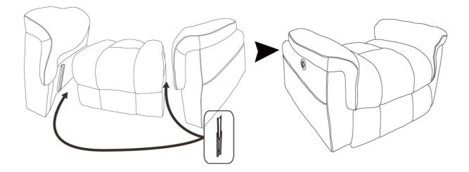
• STEP 3: Insert Chair Back (B) to the Chair Seat (A), make sure the slots on the back fully assembled to the bottom part.
