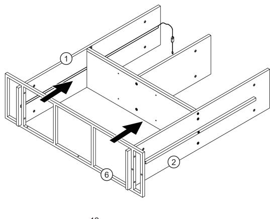
Secure the left frame (6) to the top panel and bottom panel.
