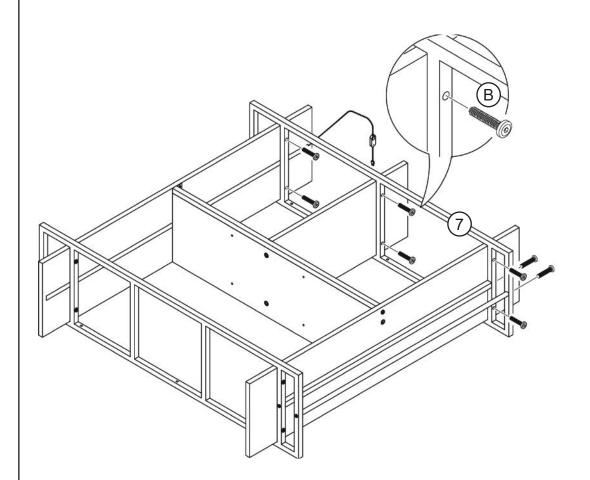
Flip the rack around, and place it front side down. Then insert wood dowels to the back of the rack.
