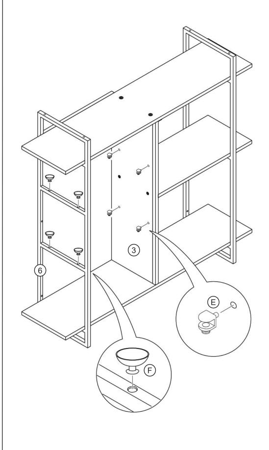
Mark the drill hole positions on the wall using the rack as a template. Make sure the rack is leveled.
