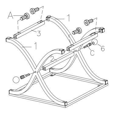
Attach Bottom Stretchers (3) to Side Panels (1) using Screws (A) and attach Center Stretcher (2) to Side Panels (1) using Screws (C).
