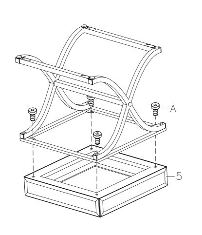
Attach the assembled metal base to Mirrored Top (5) using Screws (A) as shown.
