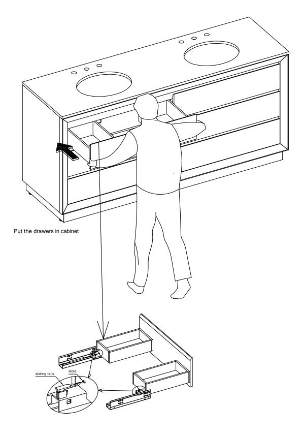
Insert the drawer by aligning the position of the slide locating pin and the hole behind the drawer as shown, then push the drawer in.
