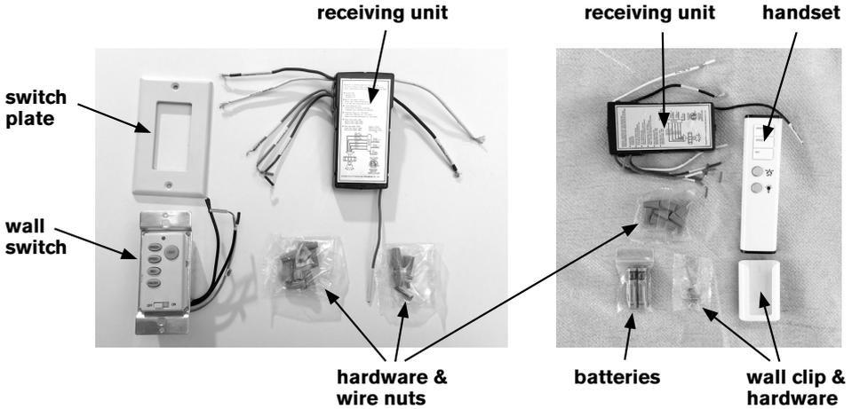
Insert receiving unit into the top of the fan body and make wire connections according to wire colors, labels and diagram below. If ordered, install wall switch into wall box, taking note of dip-switch settings and related instructions referenced below.
