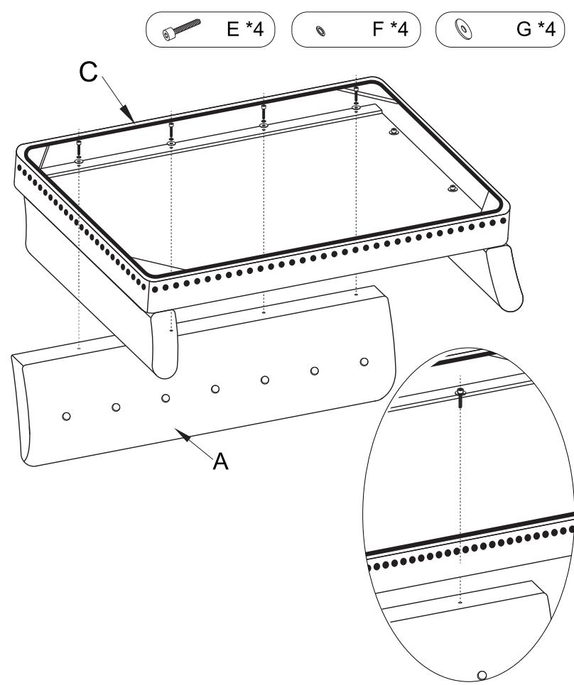
Please note that when assembling the Part C and B, firstly insert the screws through the holes of Part C until you see the threads, then align them with the holes of Part B, finally tighten the screws
