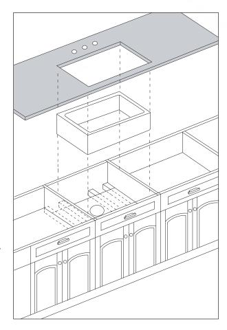
Once it is agreed upon, cut countertop accordingly. After centering the sink and allowing for any faucets and backsplashes, use a pencil to outline the sink as your guide for the cutout, allowing for any reveal before the actual cutting.
