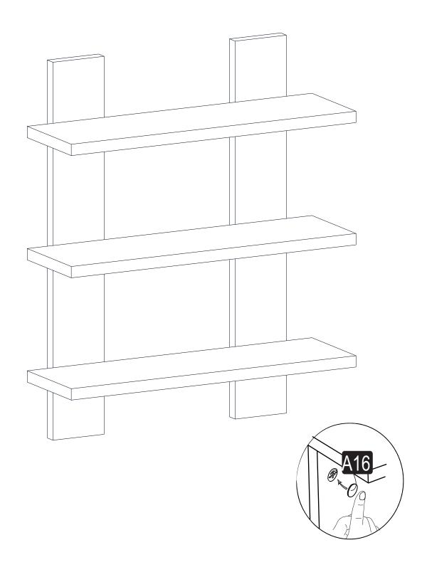
IMPORTANT; The screw supplied with the anti-topple bracket is to be used only for fixing the anti-topple bracket to the furniture. In addition, you will need to choose a screw or fitting which is suitable for securing the bracket to the type of walls you have. If you are unsure about what type of screw to use, contact your local hardware store.
