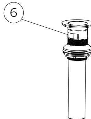
**⚠ Note:** This faucet has been packaged with an over-flow pop-up drain. **DO NOT** use with a non-over-flow sink.
