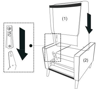
Slide the metal brackets on back cushion (Part 1) into the metal glides on seat frame (Part 2). Lower the back cushion onto the seat frame until it locks into place. Pull down the fabric flap and using the hook and loop system.
