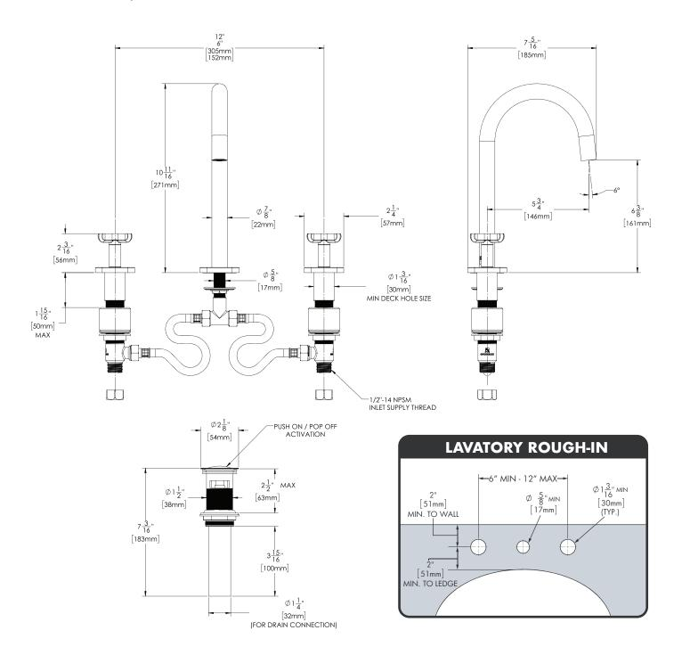
1. All dimensions are in inches (millimeters) unless otherwise specified and are subject to change without notice. 2. Contractor to supply necessary inlet connections.
