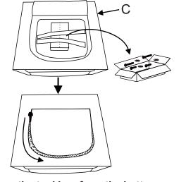
Remove the tool box from the bottom of the seat and zip it up.
