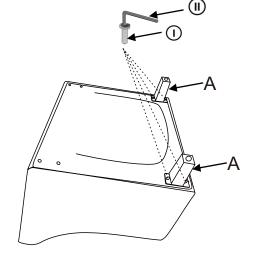
Install the front foot to the bottom of the seat.
