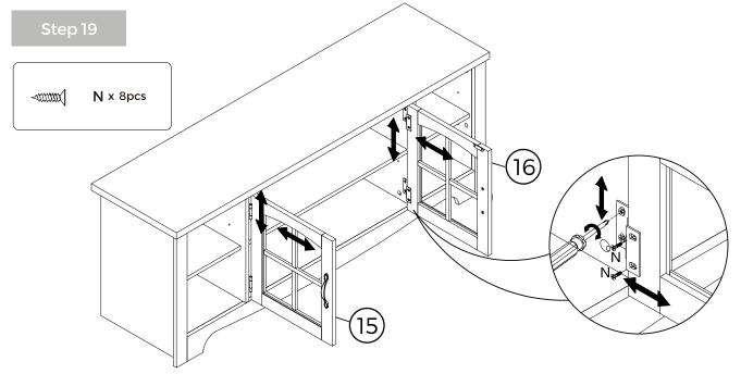
When installing the door panels, you may need to adjust the fittings according to the diagram to ensure the proper opening and closing of the door panels.
